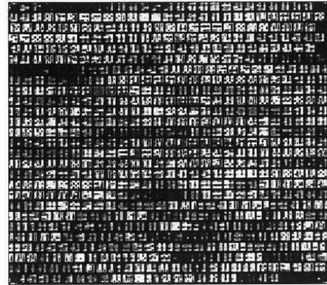
Figure 10 Fluorescent signature of hybridization array for HIV virus assay [21]. The pixels are 20-50 μm wide.
